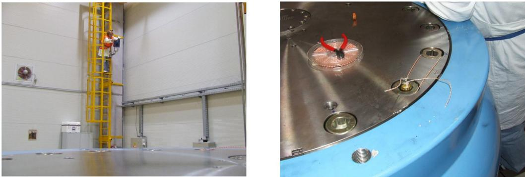
**Figure 9. Surveillance of the loading hall with an IAEA camera and sealing of the containers with common seals**
