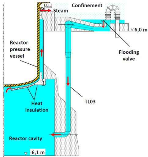
*External cooling of the reactor pressure vessel*
