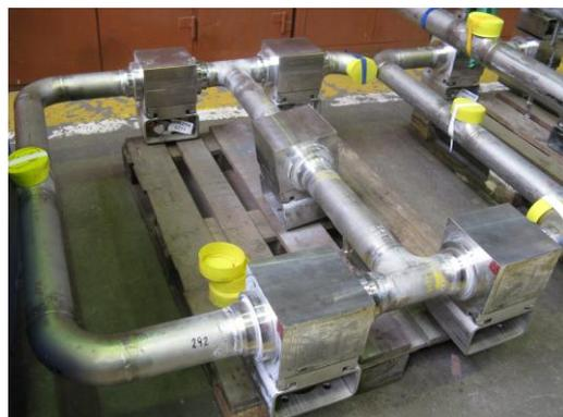
*Assembled part of the blow down system in the workshop before the tightness test of the valves*
