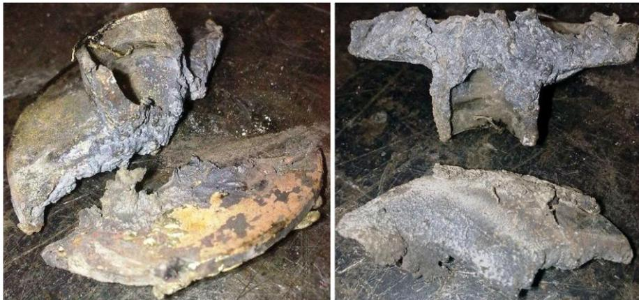
*Fractured valve plug*
